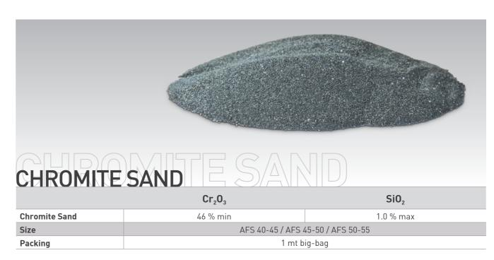
The high specific gravity and high thermal conductivity of chromite provide a pronounced chilling effect. Chromite sand has a glossy black appearance. Chromite is generally used for steel casting to provide chilling. It is difficult to reclaim chromite sand since, if it becomes contaminated with silica, its refractoriness is seriously reduced.
